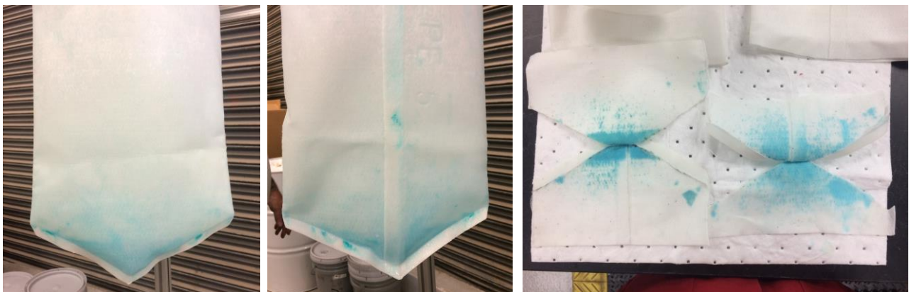
Figure 3 – Visual indication of quantity of SAP migration from the elements from Manufacturer A (SAP particles/gel dyed blue, collected in bag filters from test rig)
