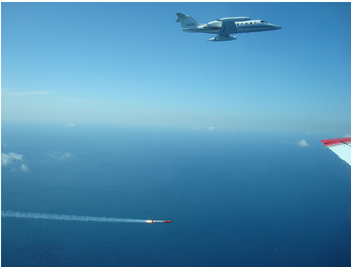
A Phoenix Air Learjet towing a simulated anti-aircraft missile used in the development of various anti-missile defenses.
