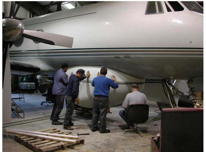
Phoenix Air maintenance specialists installing a radome on the belly of a Gulfstream G-I for use in electronic warfare training services Phoenix Air provides to the military.
