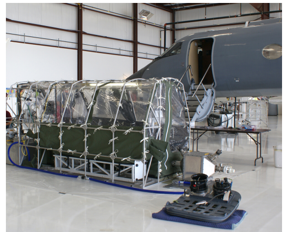
The Phoenix Air designed Aeromedical Biological Containment system and its components ready for installation inside one of Phoenix Air's highly modified Gulfstream G-III jets.
