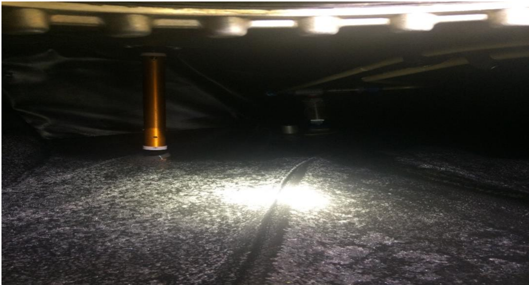
Figure 3: DEF crystallization in aircraft fuel tank.
