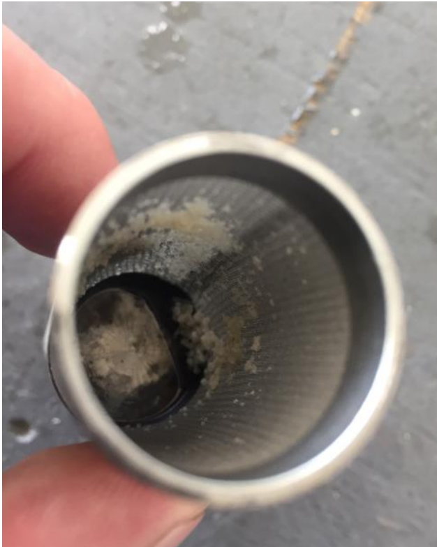
Figure 1: DEF crystallization on aircraft fuel screen.
