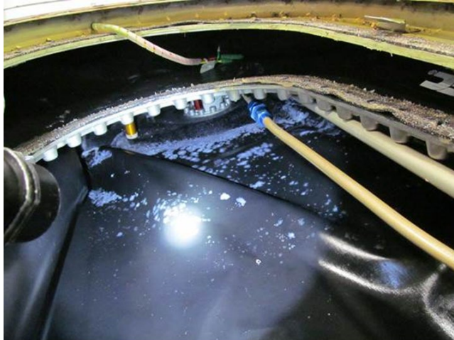
Figure 1. Auxiliary Fuel Tank with DEF Deposits
