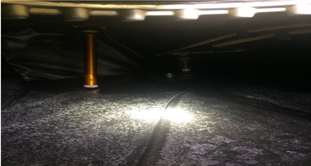
Figure 2: DEF crystallization in aircraft fuel tank.
