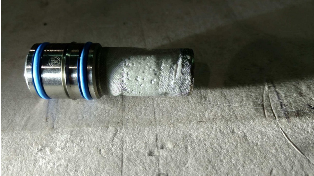
Figure 1: DEF crystallization on aircraft fuel filter.
